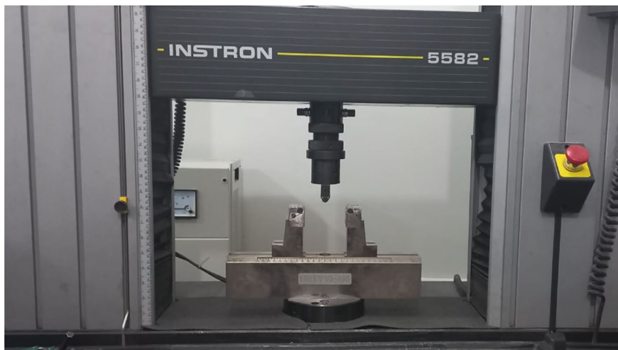
Fig. 3 Universal testing machine INSTRON model 5582. Flexural configuration
