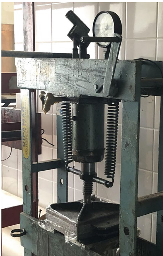
Fig. 2 Matrix under pressure during the making of the plates
